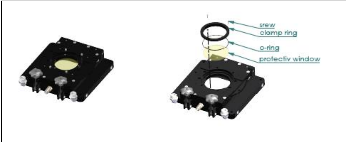
Figure 26: Change of the protective window
