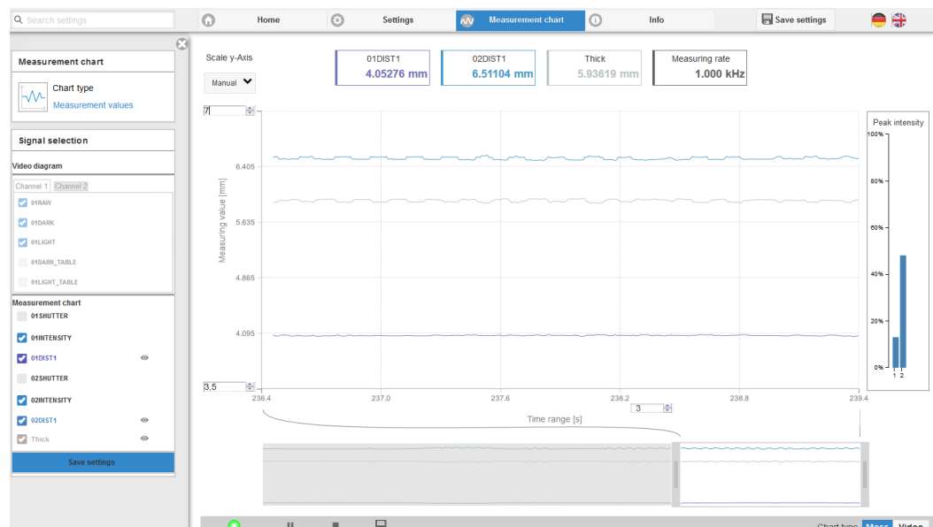
Fig. 81 Results from two-sided thickness measurement using two sensors
