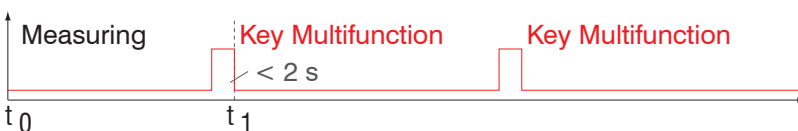
Fig. 65 Flow chart for zeroing, mastering (key Multifunction)
