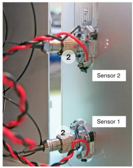
Have the new cover module with the light source on hand. Check the fiber connection of the controller for contaminations. If necessary, clean the fiber connection with a lens cloth and alcohol.
