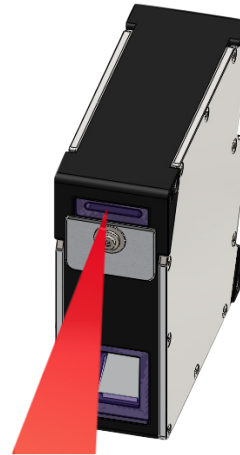
Fig. 8 Sensor with open beam attenuator for measurements
