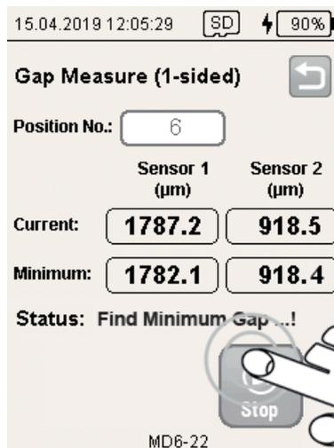
The minimum reached between **Start** and **Stop** is displayed in the **Minimum** field.
