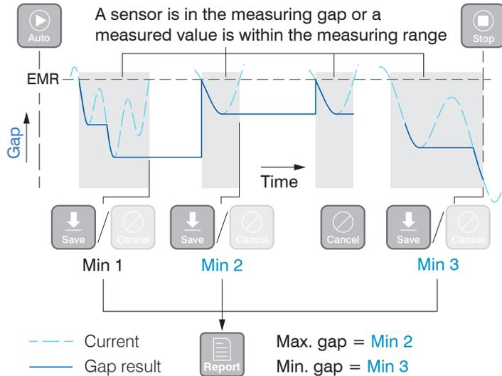
The Automatic gap detection program determines local minimums during an analysis period if a sensor is in the measuring gap. An analysis period
