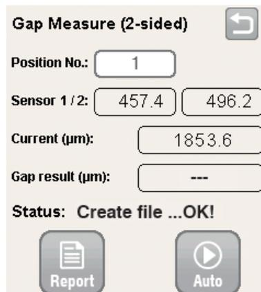
The controller starts the measurement.
