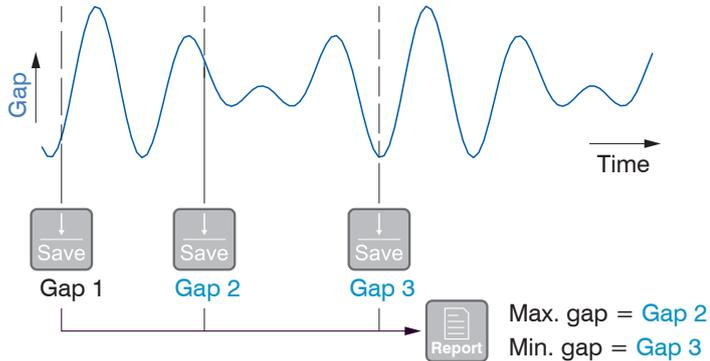
The Instant measurement program immediately saves the current measured value.
