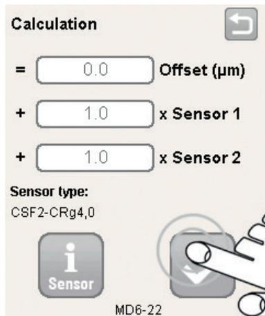
The two sensor signals can be calculated at will using a mathematical function.
