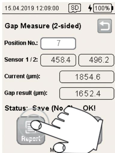
The `Gap result` field displays the smallest gap width.
