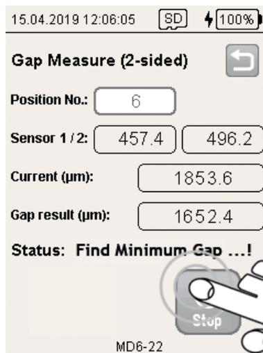
The minimum reached between **Start** and **Stop** is displayed in the **Gap result** field.
