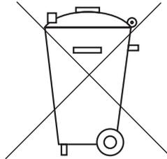
If the batteries and accumulators contain pollutants, the chemical name of the corresponding pollutants is located under the symbol of the crossed garbage can. Examples are:
