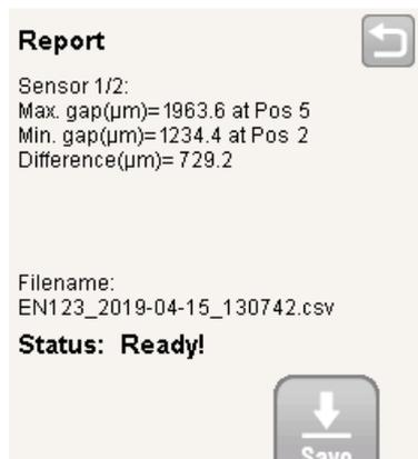
The report lists the minimum and maximum values in a series of measurements for both sensors.
