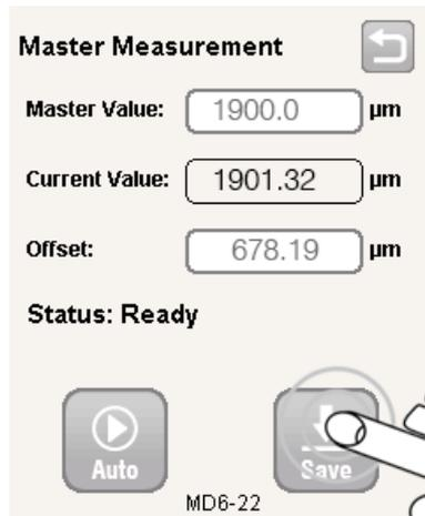
The controller calculates the actual thickness of the sensor based on the distance values and the value of the reference gap width, and displays this thickness in the *Offset* field.
