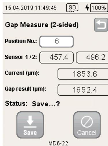
The measurement is stopped automatically, if one measured value of both sensors becomes 1% larger than the end of the measuring range.
