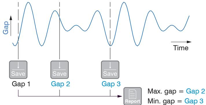
The Instant measurement program saves measured values. The Report function determines the smallest (Min. gap) and largest (Max. gap) gap width based on the derived values.
