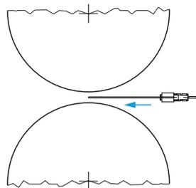
➔ Insert the sensor into the gap.
