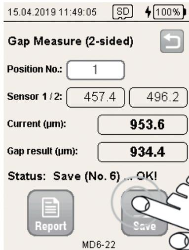
The controller measures the gap width and displays the values in the **Current** field.
