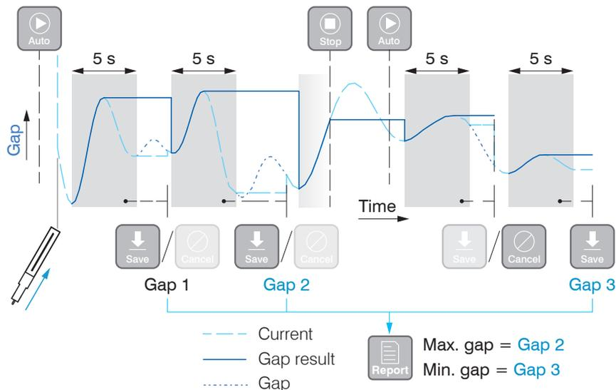
The Automatic gap detection program helps to perfectly align the sensor and determines local maximums during an analysis period.
