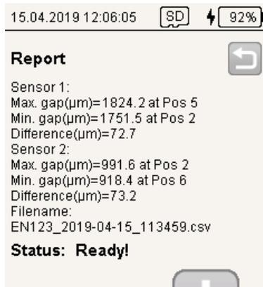
The report lists the smallest (Min. gap) and largest (Max. gap) gap width in a series of measurements for the sensor.
