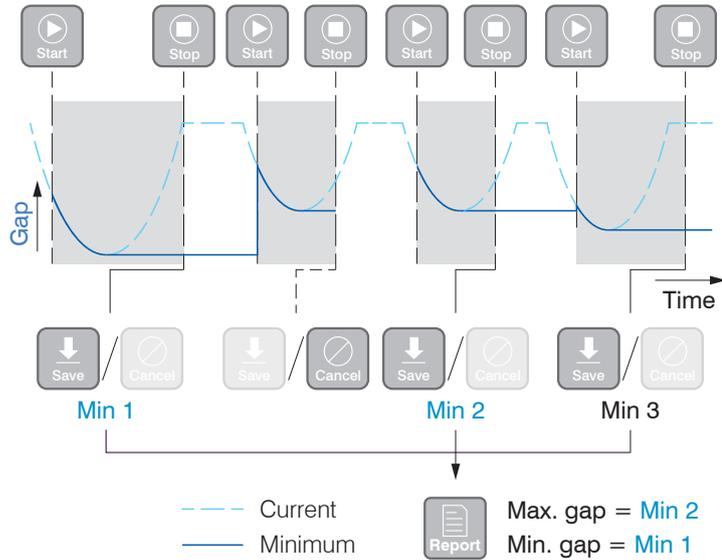
The Manual gap detection program determines the local minimum during an analysis period between Start and Stop. The Report function determines the smallest (Min. gap) and largest (Max. gap) gap width based on the derived values.
