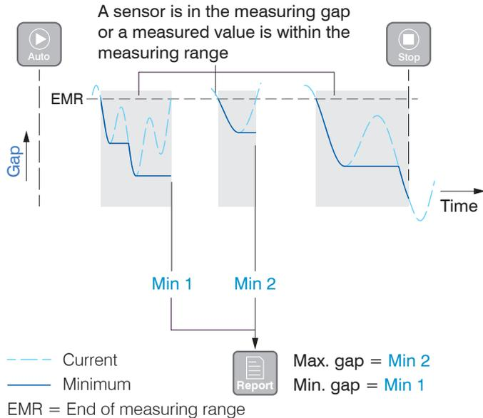
The Automatic gap detection program determines local minimums within a range between Auto and Stop if
