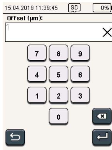
➔ Enter the thickness of the sensor used in the **Offset** field.
