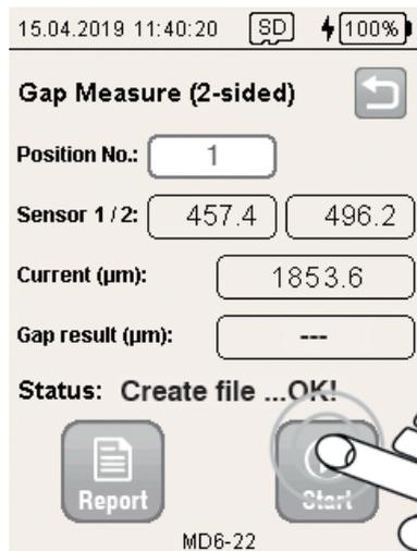
The controller measures the gap width and displays the value in the **Current** field.
