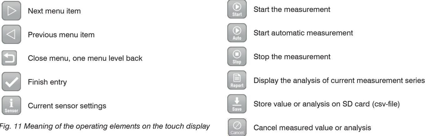
Fig. 11 Meaning of the operating elements on the touch display
