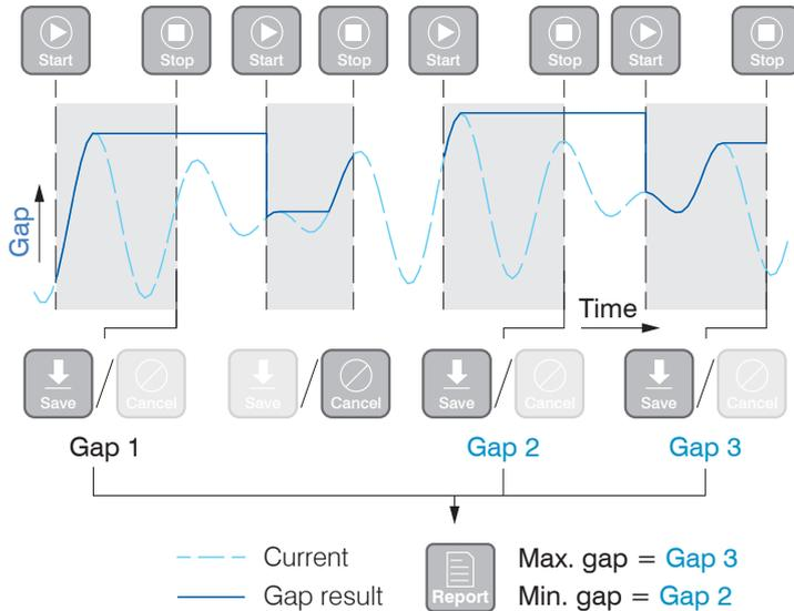
The Manual gap detection program determines the local maximum during an analysis period between Start and Stop.<sup>1</sup> The Report function determines the smallest (Min. gap) and largest (Max. gap) gap width based on the derived values.
