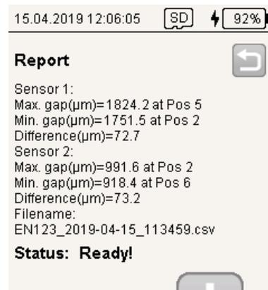
The report lists the smallest (**Min. gap**) and largest (**Max. gap**) gap width in a series of measurements for both sensors.
