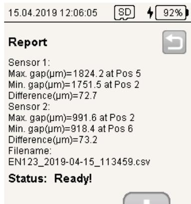
The report lists the smallest (Min. gap) and largest (Max. gap) gap width in a series of measurements for both sensors.
