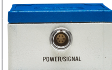
Fig. 20 Connection power supply
